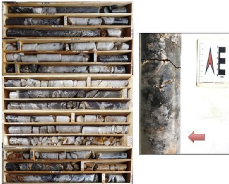
Figure 4: Drill core from Meridian drill hole DDH_BF_0004, illustrating oxide-sulphide mineralization with a package of quartz veins, 103.9 - 115.9m (example arrowed to the right). Assay results pending.
