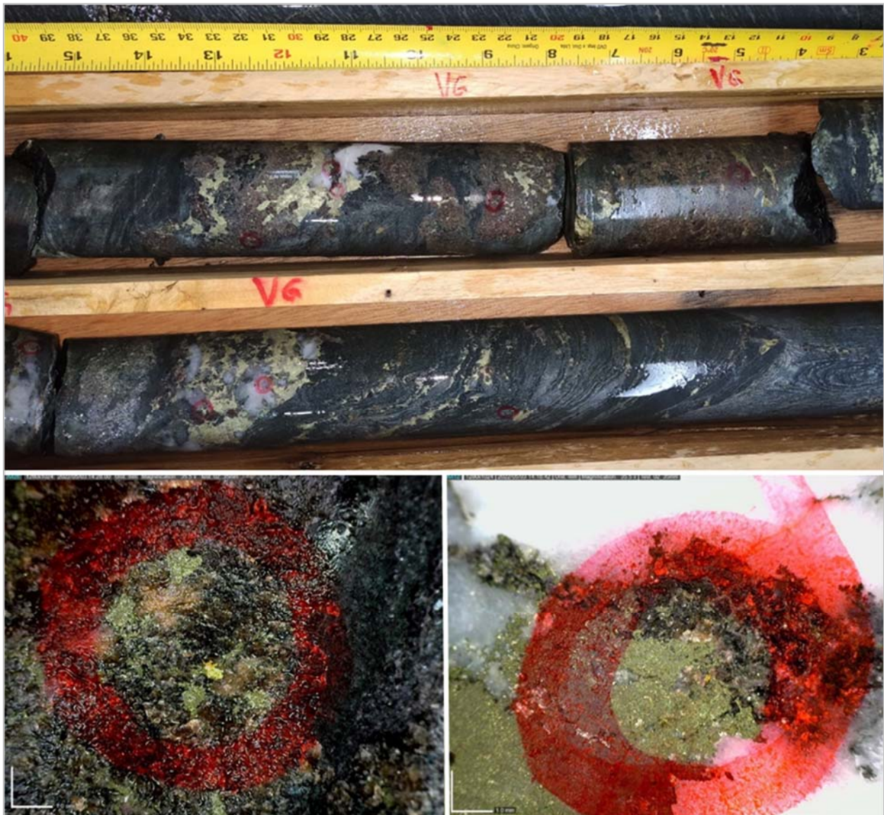
Figure 2: Top : CD-128 Visible gold (circled) within garnet-rich mine sequence host rock. Bottom : left, detail of gold within garnet matrix (red mineral), and right margin of sulphide band, in the interval 70.23m-70.53m.
