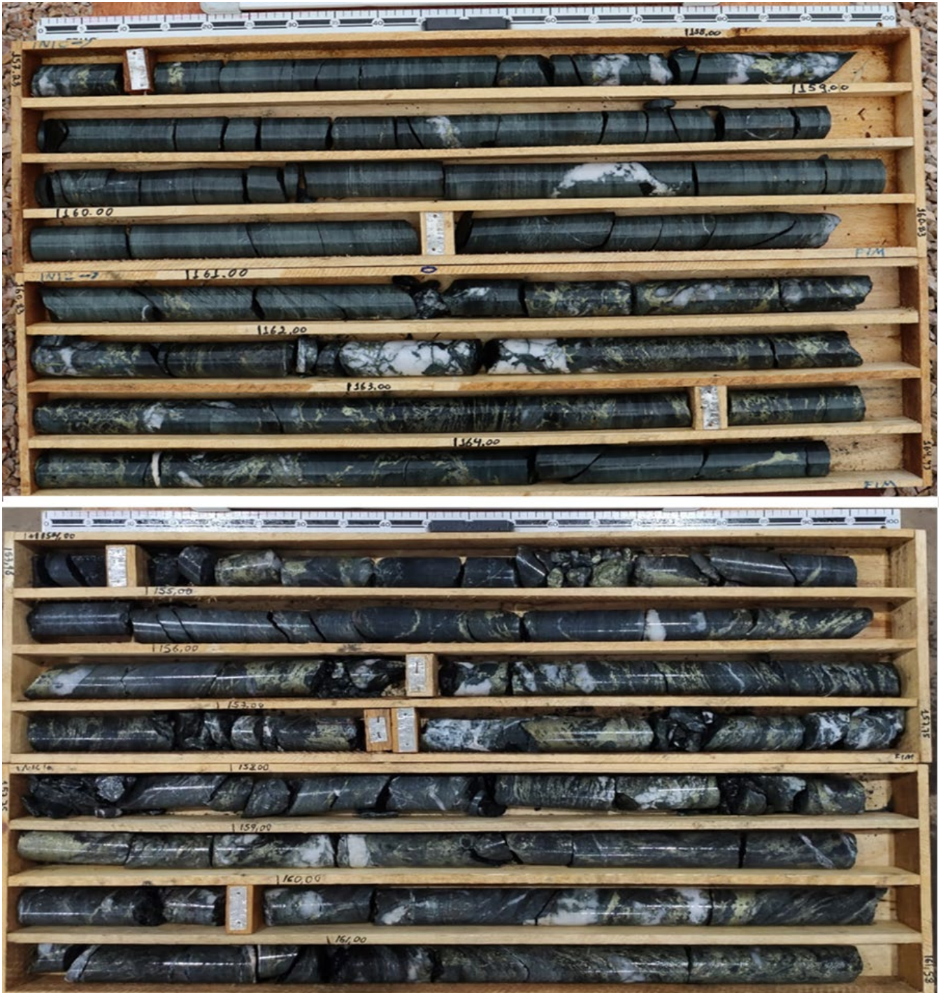
Photo 2 top: CD-003: Southern Copper Zone, Trays 47-48; 157.27 - 164.40m. Zone of stringer sulphides and quartz veining approaching sulphide breccia zone. Photo 2 bottom: CD-004: Southern Copper Zone, Trays 45-56; 153.96 - 161.68m. Zone of sulphide breccia and quartz veining.
