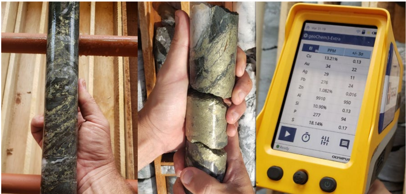
Photo 1: Left: Detail of sulphide breccia zone in CD-003. Centre: Massive sulphide vein at 119.5m in CD-004. Right: Portable XRF* analysis showing Cu-dominant assemblage with Au & Ag values and traces of Lead (“Pb”) and Zn, CD-003 breccia zone. (See below for limitations on point source readings)
