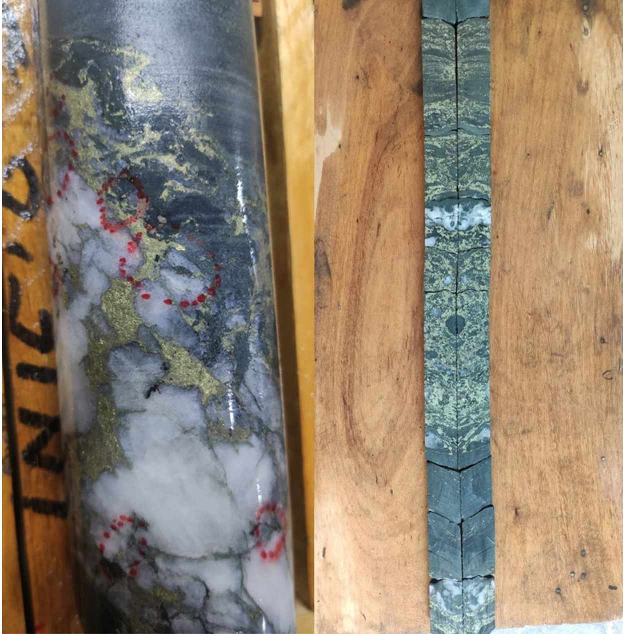
Photo 1: Left : CD-072: one of the high-grade Gold veins encountered with multiple points of visible Gold circled in red; Right : CD-070: chalcopyrite-dominant mineralization associated with strong chloritic alteration, interpreted to reflect proximity to a VMS feeder system.
