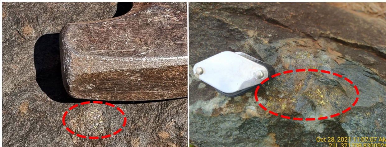
Photo 1: Examples of mineralization located in the C2A Target (Area 1 of Figure 1). Left: Example of blebby chalcopyrite-pyrite-bearing mafic rock, grading 0.4% Cu, 0.2% Zn (CBRO00027). Right: coarse chalcopyrite-dominant mineralization associated with strong chloritic alteration (assays pending).
